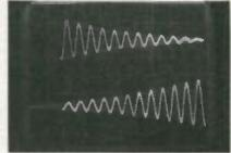
FIG. 2—AUDID OUTPUT versus horizontal position. The top waveform in this photograph is the audio signal fed to the left ear as the scan moves from left to right. The bottom waveform is fed to the right ear.
