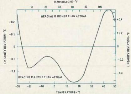
FIG. 10-TO CORRECT FOR NONLINEARITY ERRORS on the -30-+50 C range, use this curve.
