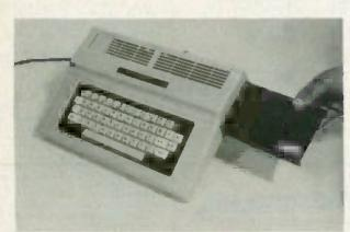
THE J & M SYSTEMS COCO DISK CONTROLLER plugs into the cartridge slot of the Radio Shack Color Computer. It works with either the old or the new models.
