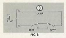
Incidentally, you may have wondered how two switches are wired so that each has complete control over a single light. The answer is to use two SPDT switches connected as shown in Fig. 6. You should be aware, however, that electricians don't call them SPDT switches, they call them "three way" switches. (So, if you need a replacement for that type, you know what to ask for!)
