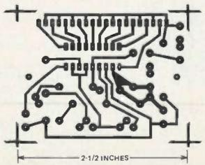
FIG. 2—THE FOIL PATTERN for the bargraph voltmeter is shown full size. The circuit layout is not critical, so you may prefer to use point-to-point wiring. But a PC board will certainly keep things nester.
