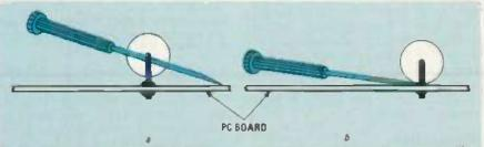
FIG. 3—SMALL JEWELERS' SCREWDRIVERS are ideal for component salvaging operations where prying is necessary: In a the screwdriver is placed between the body and lead of the unit; in bit is place under the body itself.
