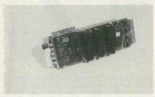
OPEN, THERE'S NOT MUCH TO SEE. A few IC's that do the electronic switching and an AV-6250 for the IEEE I O.
