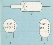
FIG. 2—TANTALUM CAPACITORS come in variety of shapes and sizes: a shows a tubular type; a disc type is in b, and c is a teardrop shaped
