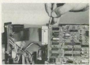
IF THE DISK DRIVE'S PRINTED CIRCUIT BOARD has holes drilled opposite the #1 and #33 terminals, pass a length of insulated #20 or #22 solid wire through the holes and around the ribbon connector. A couple of twists secures the wire and the connector.
