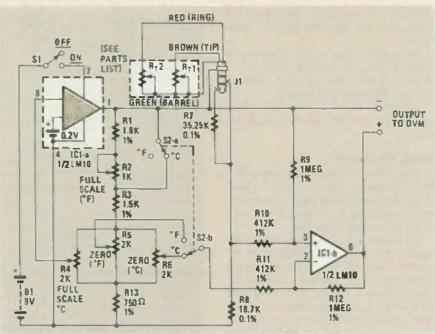
FIG. 5-THIS SLIGHTLY MODIFIED CIRCUIT measures from -30-+50 C.
