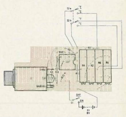
FIG. 7—CIRCUIT-BOARD ASSEMBLY using a "universal circuit board." Most of the fixed resistors must be "hairpinned" and stood on end to fit in the space allowed. Cut pin 5 from ICI—It's not needed, and a jumper is installed in its position. Note that top-side and bottom-side jumpers are shown. Those on the bottom are shown dashed. Solder R7 directly between the ring and tip of J1 before gluing the lack to the board.
