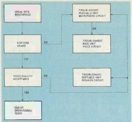
FIG. 7—THE VOICE TEST is the final check to be performed. Drice all of the tests are performed, it is possible to troubleshoot and repair the telephone.
