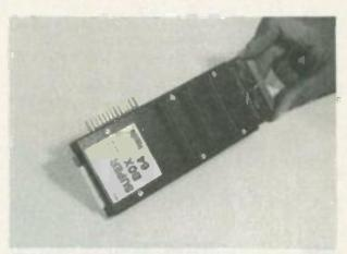
THE SUPER BOX 64 is a complete three-cartridge switching system an IEEE VO for the Comodore 64.
