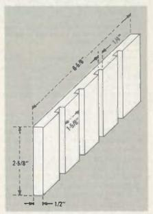
FIG. 9—DEMENSIONS FOR the side panels of the parts box is shown here.
