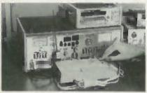
FIG. 8—USING AN FM DEVIATION METER to measure FM modulation. For a cordiess phone, 3 to 4 kHz of deviation should be seen during the ring signal.
