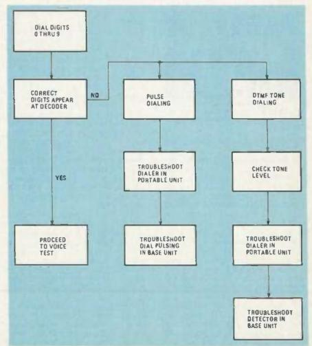
FIG. 6-TO DETERMINE If there is a problem with the telephone's dialing system, this test should be performed.
