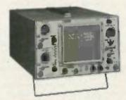
FEATURES • 1 mV/div sensitivity • 20 calibrated sweeps • Rectangular CRT with internal graticule and scale liturnination • Video sync separators • X-Y operation • Z axis input • 6kV accelerating voltage • X10 sweep reagnification • Auto sweep • Vmode-displays two signals unrelated in frequency • Sum & differ-
