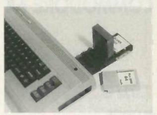
THE SUPER BOX 64 PLUGS INTO THE USER PORT on the back of the Commodore 64. The program cartridges are then plugged into any of the three ports on the Super Box. The edge connector sticking out is the IEEE I O. Mounting feet on the bottom of the unit raises it to the same height as the computer so everything sits flat on the table.
