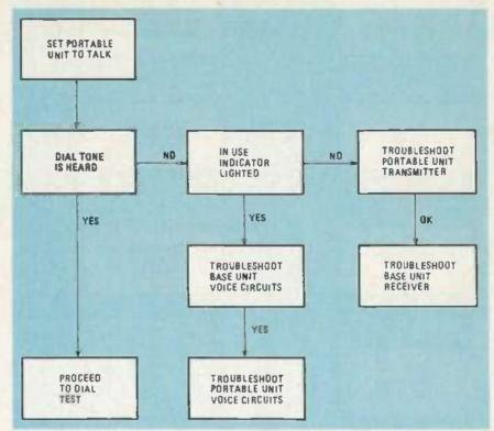
FIG. 5—EVEN IF THE RING TEST should uncover a fault, the disistone test should be performed
