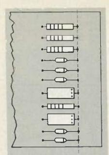
FIG. 7—CIRCUIT BOARDS can be easily stripped using this brute-force method when components are sligned.
