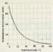
FIG. 1—A SINGLE THERMISTOR has a highly nonlinear realistance-val-temperature characteristic.
