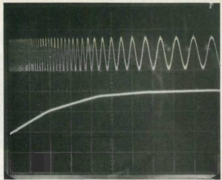
FIG. 3—HEIGHT INFORMATION is coded by changes in frequency. The top waveform shows the frequency change as the scan moves from top to bottom. That waveform is generated in response to the signel shown in the bottom of the photograph.
