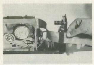
WRAP TWO TURNS of friction tape around the ribbon wire to protect it where the disk drive's cabinet and the rear panel meet.
