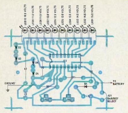
FIG. 3—PARTS PLACEMENT DIAGRAM. Note that for the unit to read from left to right, it must be installed foll-side up.
