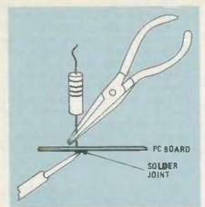
FIG. 4—NEEDLE NOSE pliers holding the component lead double as a heat sink to prevent possible thermal damage.
